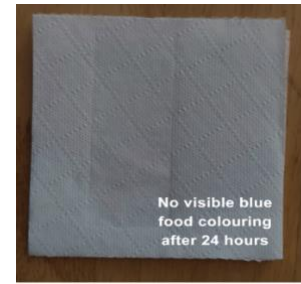
Figure 13 – Validation of PETG HF watertightness with basic print settings: Test outcome
