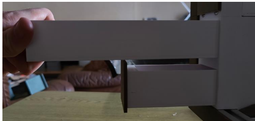
Figure 16 – Drawer, top 0.2mm clearance, bottom 0.3mm clearance
