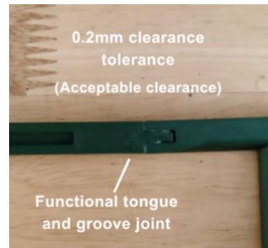
Figure 15 – Tongue & groove joint, 0.2mm clearance
