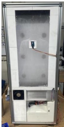
Figure 34 - Back of the machine showing the root chamber, with the misting chamber on top and pump compartment at the bottom.
