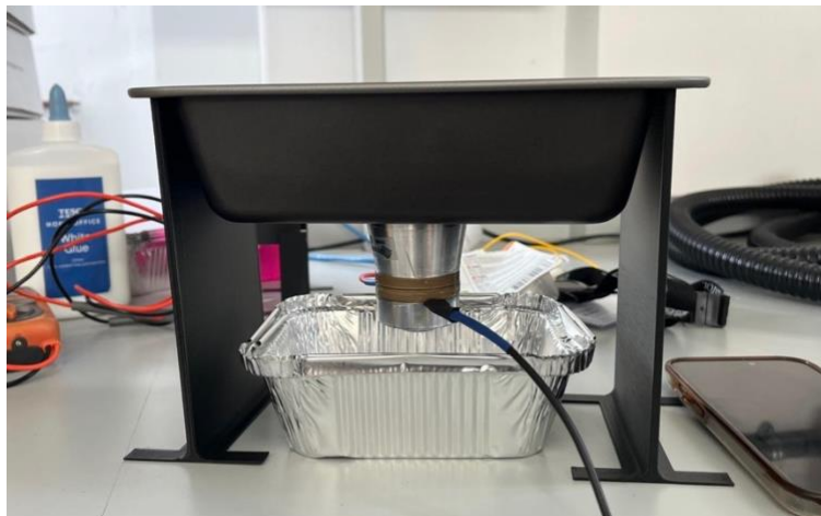
Figure 20 - Transducer glued to metal tray
