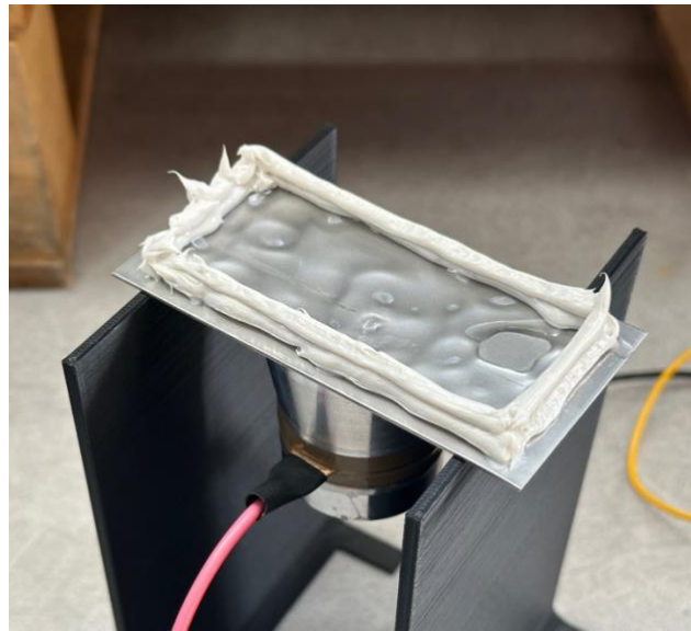
Figure 22 - 3rd setup when transducer was generating 40kHz frequency
