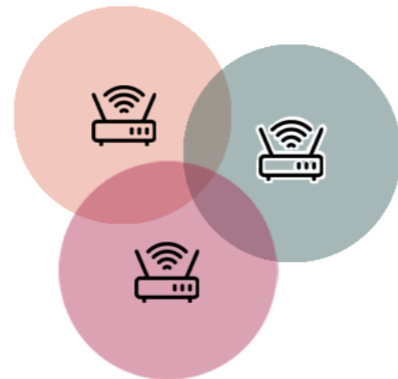
Adjacent-channel Every client and access point on overlapping channels talk over each other
