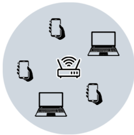
Co-channel Every client and access point on the same channel competes for time to talk
