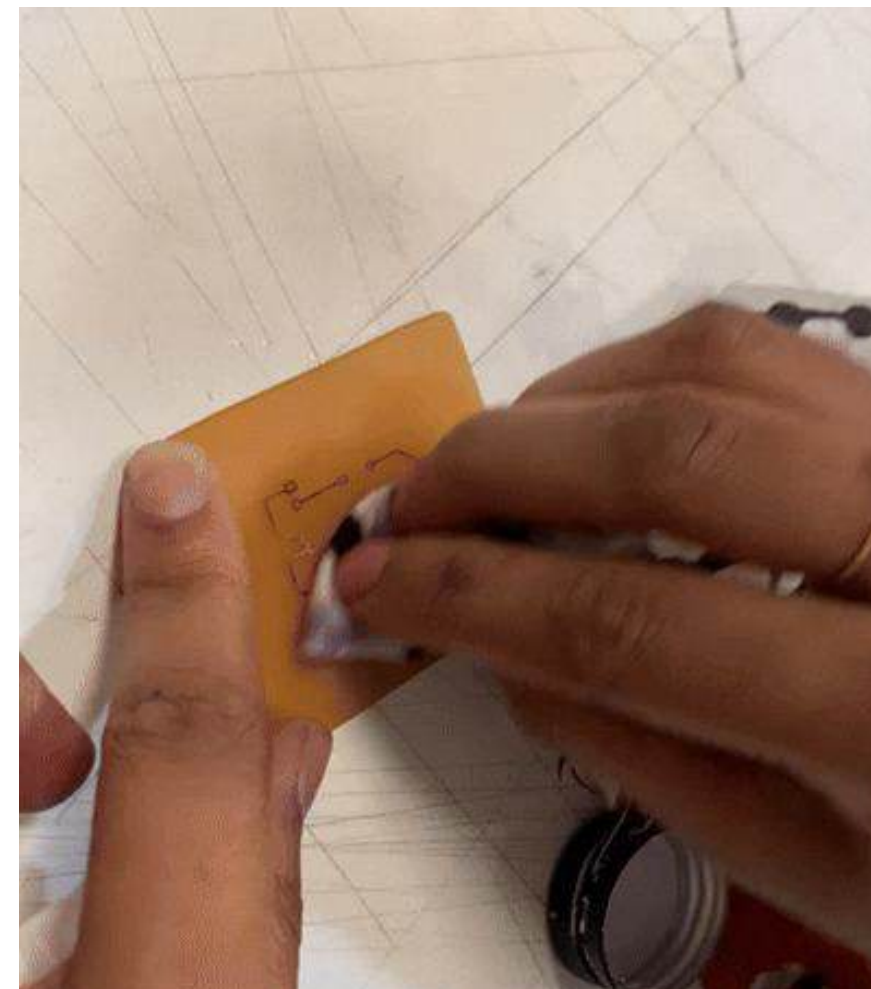
Submerge the copper-clad board in the solution, agitate for about 10 minutes until the copper fades to yellow, wash it and then use thinner to remove the black lines.
