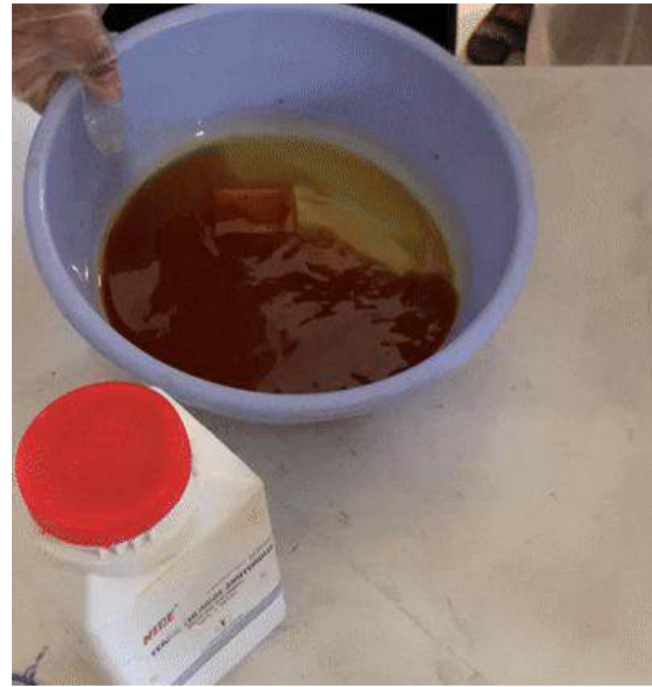
Submerge the copper-clad board in the solution, agitate for about 10 minutes until the copper fades to yellow, wash it and then use thinner to remove the black lines.
