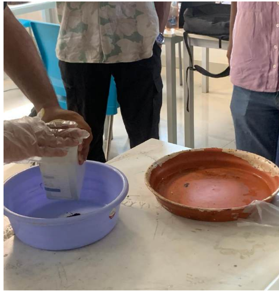
Ferric chloride anhydrous with water in 1:1 concentration and mix properly.
