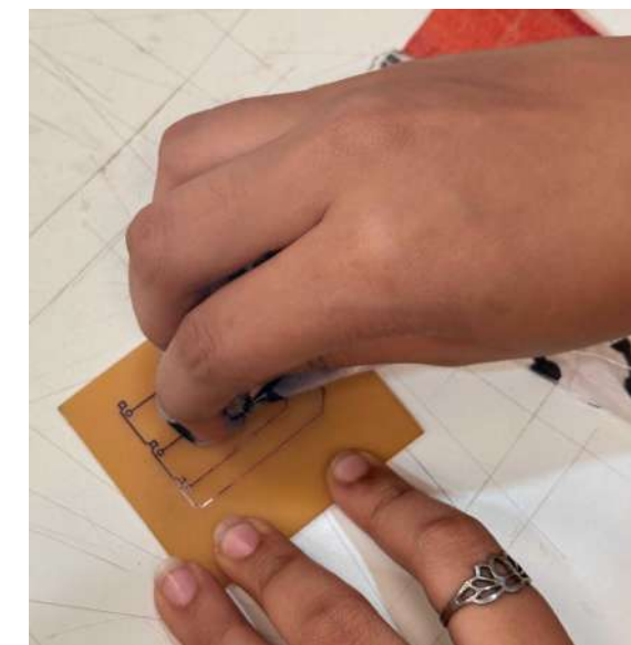
it is cleaned with thinner and copper will be visible
