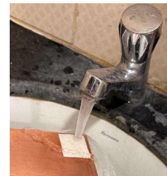
Washing – The board is cleaned with water to remove excess paper.
