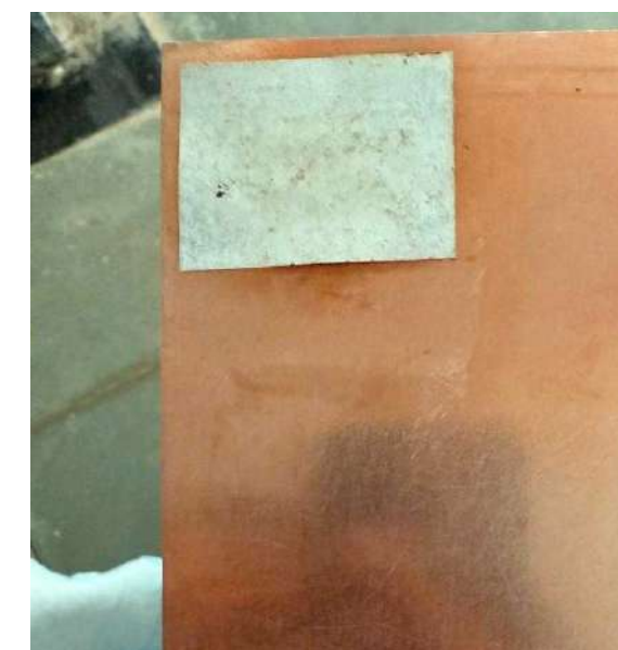
Printing & Transfer – The PCB layout is printed and transferred onto the copper board.
