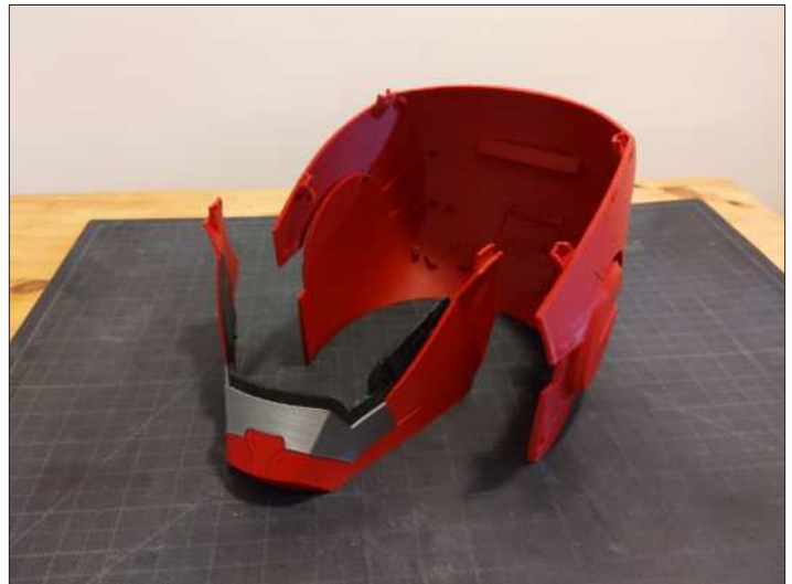
Step 12. Use two m2x4mm bolts to attach by the left cheek.
