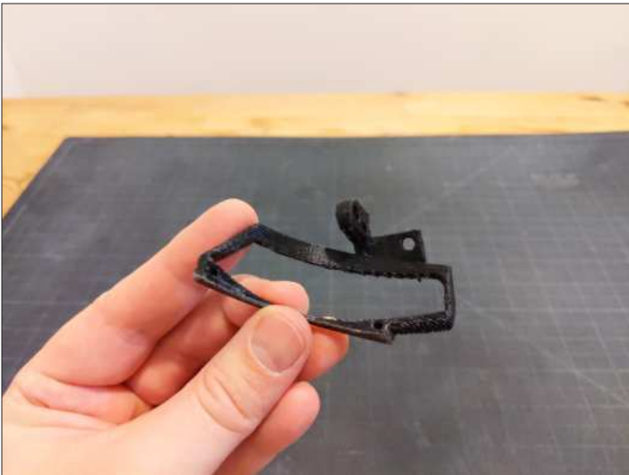
Step 125. Align led panel as shown and mark for those two holes.
